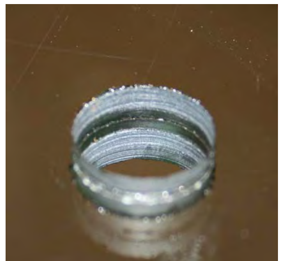
Hole made using keyhole saws for CNC. Pls. note the minimum chipping and the PVB which is not so much torn and well cut.
